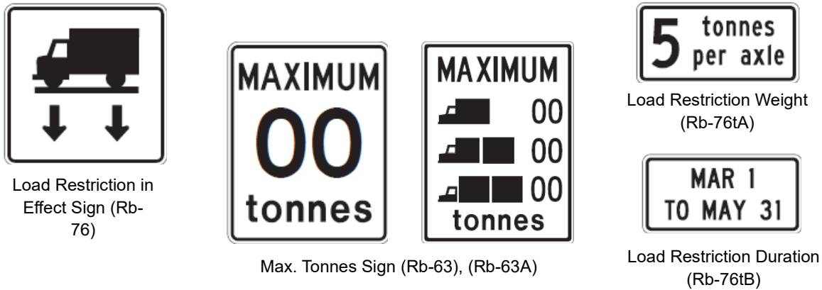
Figure 2: Load Restrictive Signage
